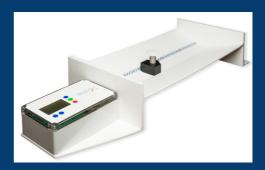
An industrial linear position sensor is used to provide a highly linear and repeatable length measurement and data is transferred automatically via RS232 cable or Bluetooth when a sample is taken.
